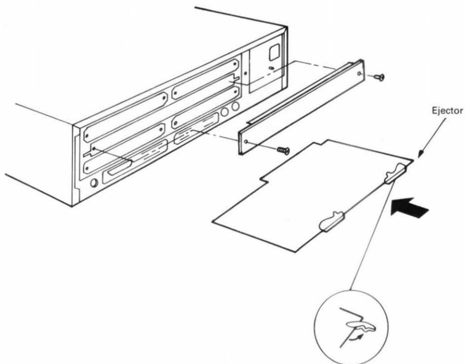
For removal, pull out in direction of arrow so that the ejectors can stay up.
